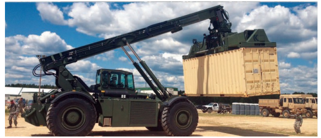
Figure 2: The RTCH with an engaged container. Note the spotters at the back and front.
