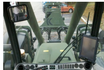
Figure 9: Touch screen, mounted on lower right in the RTCH cab.
